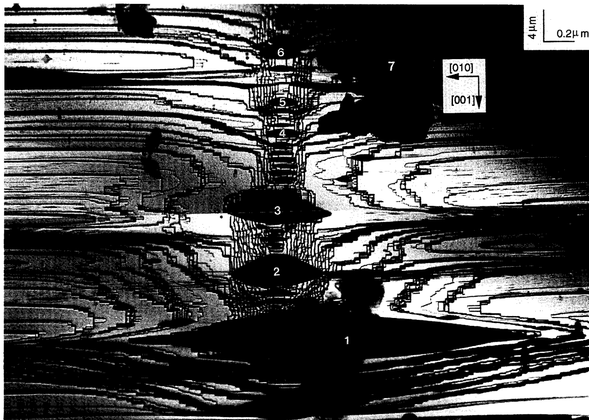
Fig. 12. A REM image of the \text{LaAlO}_3(100) surface showing the effect of the Si–La–O particles on the formation of surface steps. The image was recorded using the (1000) specular reflected beam under the diffracting conditions shown in Fig. 3a. This image is a match of two images recorded under different focusing in order to view the entire region clearly. The sharp line across particle 3 is the match line, the contrast variation across which is purely a photographic effect and has nothing to do with the structure of the surface. Particles 1–6 are the surface contaminants. Particle 7 is a fracture fragment standing on the surface.
