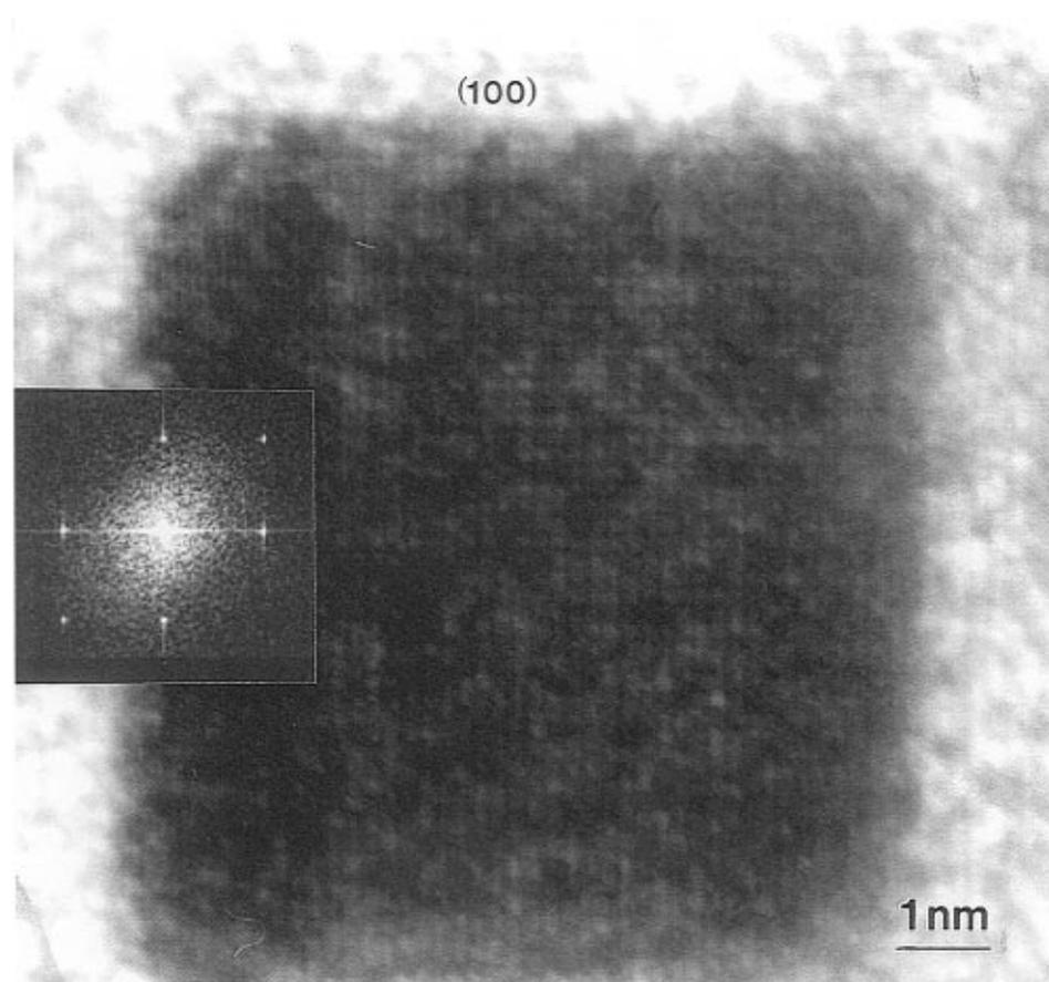
**Figure 2.** High-magnification TEM image of a cubic-shaped platinum nanoparticle showing the {100} plane. Also, the optical diffractogram of the image is shown (inset).
