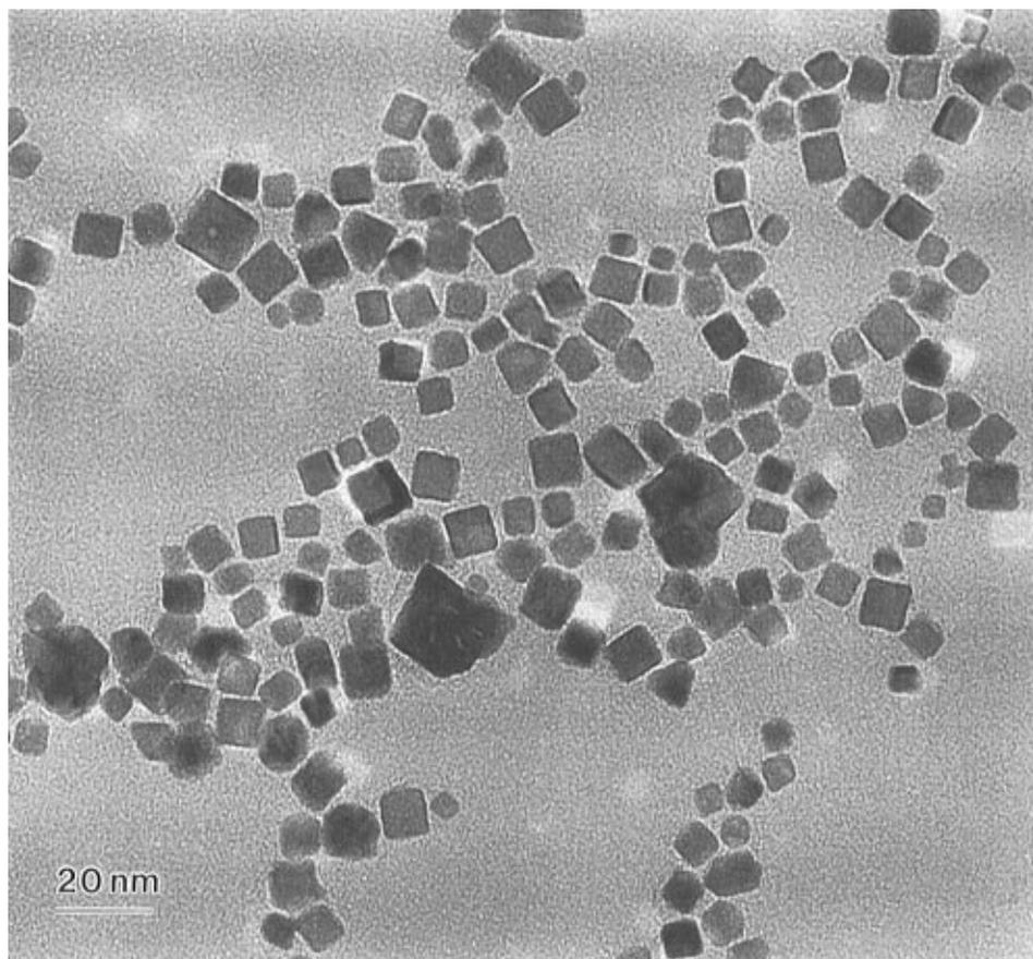
**Figure 1.** Low-magnification TEM image of the platinum particles showing the abundance of the cubic-shaped particles.
