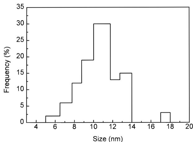
**Figure 3.** Histogram showing the size distribution of cubic Pt nanoparticles.
