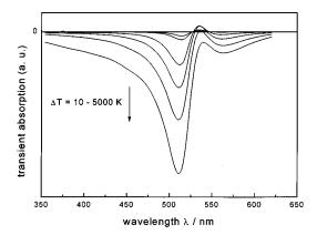
FIG. 6. Calculated transient absorption spectra for 22 nm gold nanoparticles. The temperature change  $\Delta T$  of the electron gas is 10 (displayed as  $\times$ 5), 100, 500, 1000, 2000 and 5000 K assuming a thermalized Fermi distribution. The plasmon band bleach increases and broadens with increasing temperature change.
