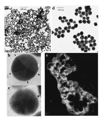
FIG. 4. Low magnification TEM image of 15 mm gold nanoparticles (a). HRTEM images of the same sample are displayed in (b) and (c). A multiple twin (b) and a stacking fault (c) can be clearly seen as indicated by the arrows. (d) and (e) show a low magnification TEM and a dark field image of 48 mm gold particles. Multiple twins and stacking faults are also present in these larger nanoparticles.
