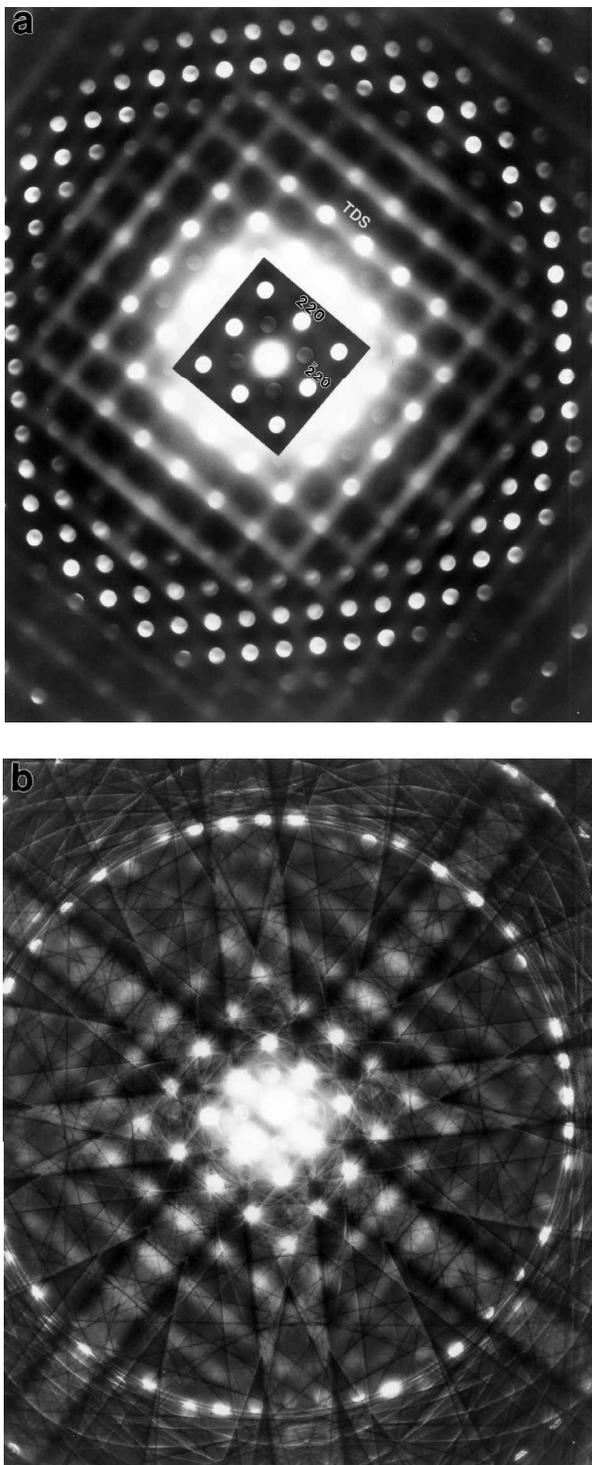
Figure 3. Experimentally observed electron diffraction patterns from (a) a thin and (b) a thick region of a GaAs foil, showing the presence of strong  $\langle 110 \rangle$  TDS streaks in the pattern.
