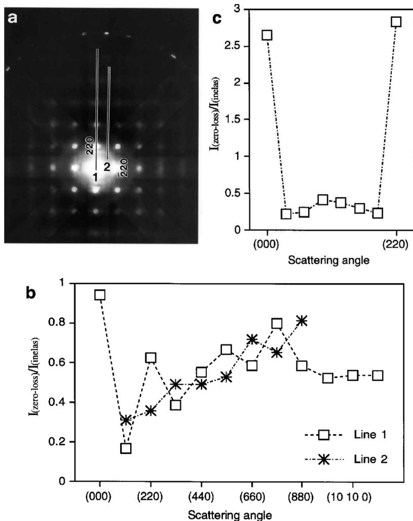
Figure 4. (a) An electron diffraction pattern recorded from Si[100]. (b) The angle-resolved intensity ratio of the total inelastically scattered electrons to the zero-loss peak measured by EELS in the diffraction mode (see text) along the lines indicated in (a). (c) The same as (b) except for a different region with finer scan between  $(000)$  and  $(220)$ . The electron voltage is 200 kV, the camera length is 1.6 m and the EELS entrance aperture size is 3 mm.
