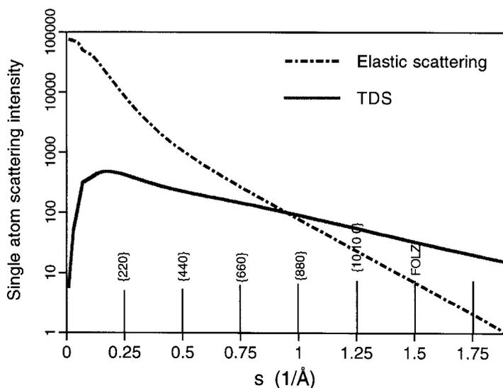
Figure 2. Theoretically calculated atom scattering factor  $[(f^e)^2 \exp(-2W)]$  for elastic scattering and atom scattering factor  $(f^e)^2[1 - \exp(-2W)]$  for the TDS of a Si atom, showing the dominant contribution of TDS at large scattering angles, where  $W$  is the Debye-Waller factor. The scattering vector  $\mathbf{s} = \mathbf{g}/2$ . The rms atomic vibration amplitude was taken as  $0.07 \text{ \AA}$  in the calculation.
