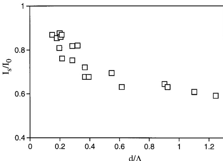
Figure 5. The ratio of the total transmission electron intensity measured by EELS in the image mode of a GaAs foil oriented along the [100] zone axis, with ( $I_s$ ) and without ( $I_0$ ) the presence of the specimen in the beam path, as a function of the specimen thickness  $d$ . The electron voltage 200 kV, the image magnification is 100 000 $\times$  and the EELS entrance aperture size is 3 mm.
