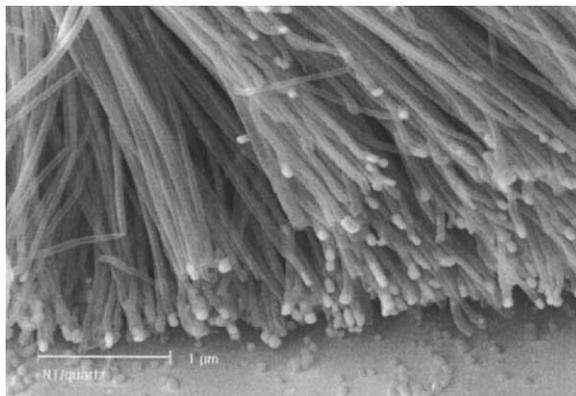
Fig. 1. SEM image of the iron particles within tips of the aligned nano tubes.
