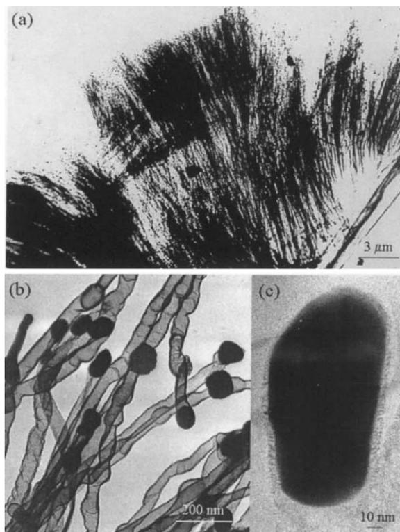
Fig. 2. TEM image of the particles and the nanotubes. (a) A bunch of the aligned carbon nanotubes; (b) top view of the aligned nanotubes, showing the large iron particles; (c) HR-TEM image of the nanotube tips.
