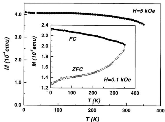
Fig. 3. Temperature dependence of magnetization in the field of 5 kOe. The inset is the magnetization as a function of temperature obtained in the zero-field cooled and field cooled process with field of 0.1 kOe.
