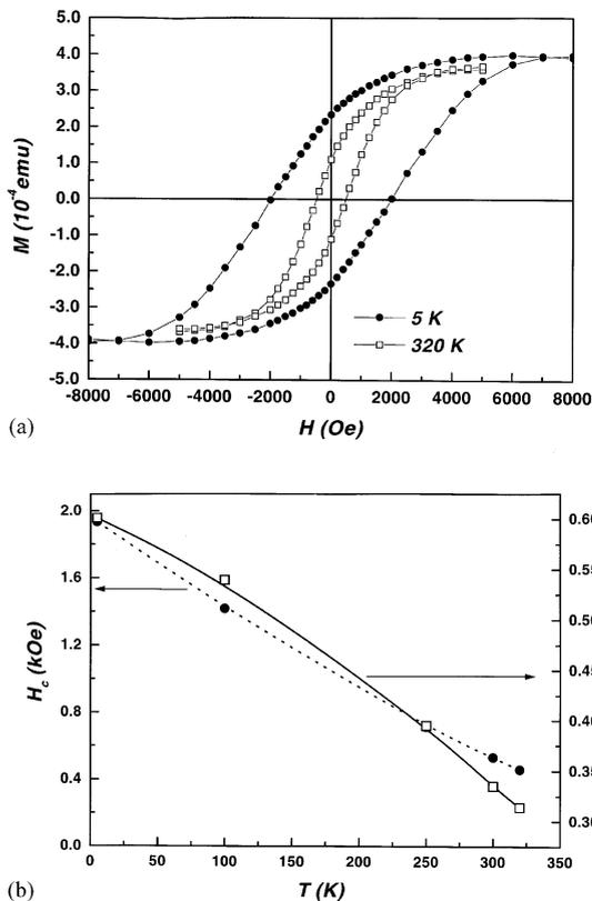
Fig. 4. (a) Hysteresis loops obtained at 5 and 320 K with magnetic field parallel to the tubes; (b) the temperature dependence of the ratio  $M_r/M_s$  and coercive field  $H_c$ .
