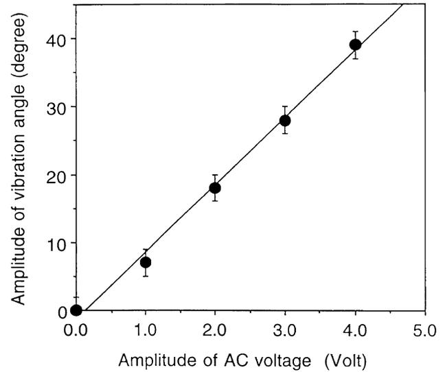
Fig. 2. Experimentally measured full vibration angle of a carbon nanotube as a function of the amplitude of the applied AC voltage.
