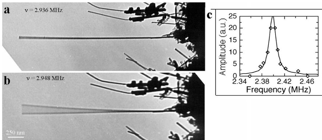
Fig. 1. A carbon nanotube produced by arc-discharge at (a) off-resonance and (b) on-resonance by varying the frequency of the externally applied electric field. (c) The full width at half maximum of the resonance peak.
