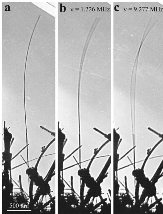
Fig. 3. A bent carbon nanotube at (a) stationary, (b) the first and (c) the second harmonic resonance induced by an externally applied electric field.
