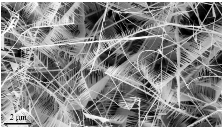
Figure 22 SEM image of comb-like nanostructure of ZnO, which is the result of surface polarization-induced growth.
