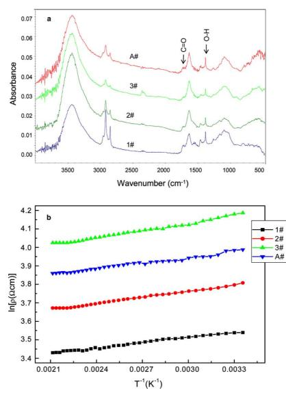
Fig. 3. (a) FT-IR spectra of the MWNTs from different samples, demonstrating the carboxyl groups binding on them and (b) the resistivity versus temperature plots for the MWNTs films.
