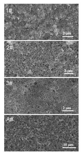
Fig. 2. Topography SEM images of the MWNTs electrodes, displaying uniform surfaces.
