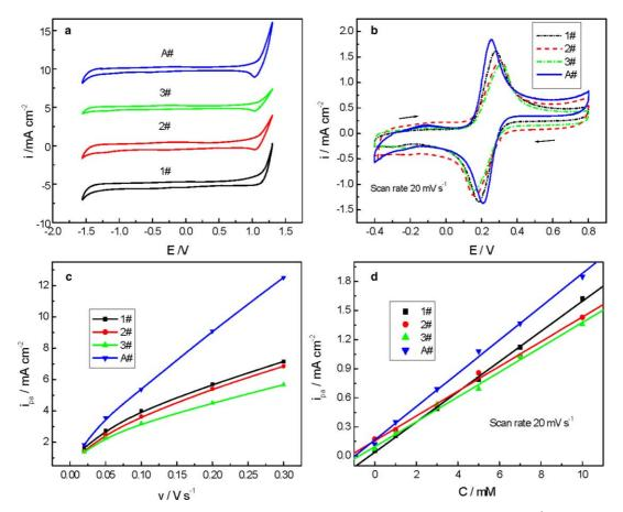
Fig. 4. Voltammetric behaviors of the MWNTs electrodes (a) potential window in 0.1 M KCl at scan rate of  $20 \text{ mV s}^{-1}$ , (b) cycle voltammogram for 10 mM K<sub>4</sub>Fe(CN)<sub>6</sub> in 1 M KCl, (c) the changes of oxidation peak current densities versus scan rate for 10 mM K<sub>4</sub>Fe(CN)<sub>6</sub> in 1 M KCl and (d) the changes of oxidation peak current densities versus concentration of  $Fe(CN)_6$  in 1 M KCl.
