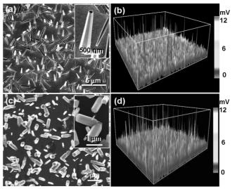
**Figure 5.** a) A typical SEM image of sparsely grown ZnO nanocones (inset: a magnified view of a single nanocone) and b) the corresponding AFM voltage output profile ( $20~\mu m \times 20~\mu m$ ). c) An SEM image of a typical top-down view of a randomly oriented ZnO NW array on a plastic substrate (inset: an enlarged view showing the randomly tilted NWs on a plastic substrate) and d) the corresponding AFM voltage output profile ( $20~\mu m \times 20~\mu m$ ).
