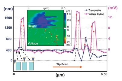
**Figure 3.** The simultaneously recorded line scanning topography image (blue dotted line) and voltage output profile (pink line) of several aligned ZnO NWs. The inset in the upper part of the figure shows a 2D height profile (top) and a simultaneously recorded voltage output image (bottom) obtained by scanning the tip across an area of 6.5  $\mu$ m $\times$ 3.2  $\mu$ m. A schematic depicting the tip and NW local contacts is displayed at the bottom left corner for the corresponding locations.
