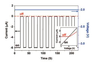
Figure 5. Current response of Device no. 4 to periodic releasingbending process under a fixed bias of -2 V, showing an "on"–"off" ratio of ~120. Inset is I-V characterization of Device no. 4 without (black curve) and with stain (red curve).
