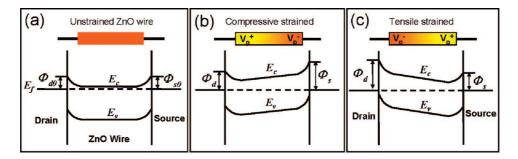
**Figure 4.** Schematic energy band diagrams illustrating the Schottky barriers at the source and drain contacts of a unstrained (a), compressive strained (b), and tensile strained (c) PFW, which illustrates the effect of switching the piezoelectric potential either by strain or by wire orientation on the local band structure and SBH.
