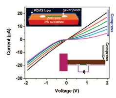
**Figure 1.** Typical I-V characteristics of the device under different compressive strains (Device no. 1). Black line is the I-V curve without strain. The direction of the blue arrowhead indicates the increase of applied compressive strain. Upper inset shows the schematic of a single ZnO PFW-based device. Lower inset shows the schematic of the electromechanical measurement system.
