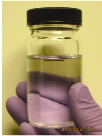
Figure 9 A digital photograph of the reaction container showing the substrate floating on the solution surface by surface tension
