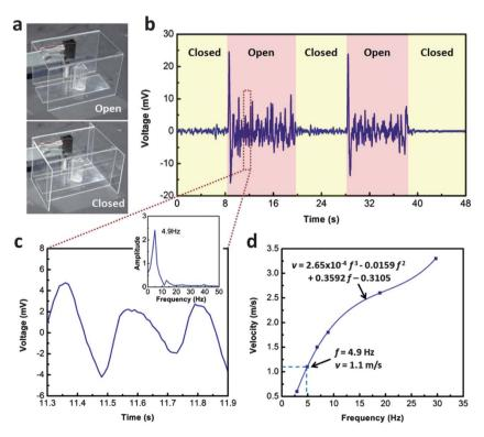
**Fig. 4** Ambient wind-speed measurement with the NG-based VFD. (a) Photos of the device with the wind passage open and closed. (b) Voltage output of the NG. (c) Magnified output curve from 11.3 s to 11.9 s. The inset shows the frequency spectrum of the output curve from 11.3 s to 11.9 s. (d) Frequency–velocity curve.
