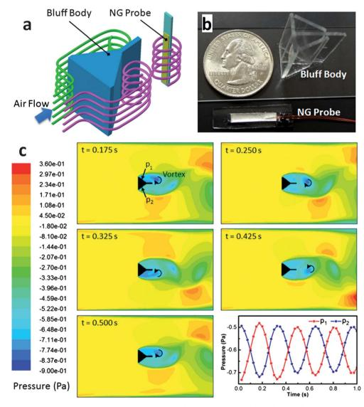
**Fig. 2** Schematic and simulation of the NG as an active sensor for detecting air flow. (a) Working principle of the vortex generation and capture. (b) Photo of the bluff body and the NG probe. (c) Transient pressure contours at different times, and curves of mean relative pressures on the two back faces.
