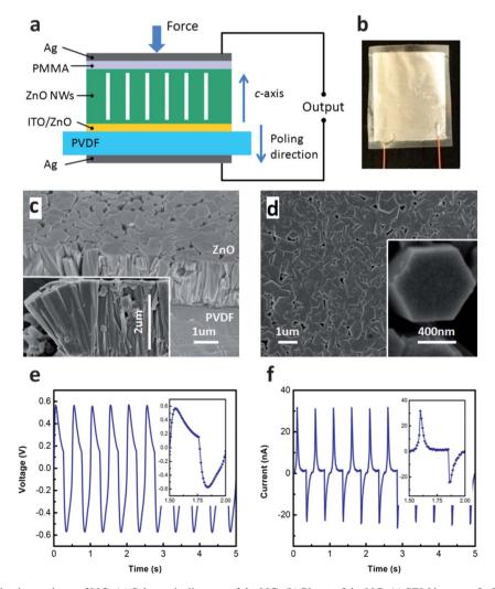
Fig. 1 Design, characterization and test of NG. (a) Schematic diagram of the NG. (b) Photo of the NG. (c) SEM images of a ZnO NWs array grown on a PVDF substrate. The inset shows a magnified cross-sectional image. (d) Top-view of the ZnO NWs array. The inset shows a magnified image of a ZnO NW. Electrical characteristics of the NG. (e) Voltage output. (f) Current output.
