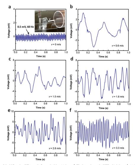
**Fig. 3** Voltage outputs of the NG under different air-flow velocities. (a)  $0 \text{ m s}^{-1}$ . The inset shows the VFD. (b)  $0.6 \text{ m s}^{-1}$ . (c)  $1.5 \text{ m s}^{-1}$ . (d)  $1.8 \text{ m s}^{-1}$ . (e)  $2.6 \text{ m s}^{-1}$ . (f)  $3.3 \text{ m s}^{-1}$ .
