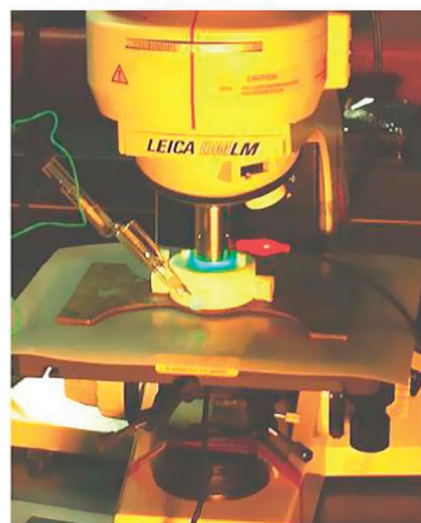
Figure 8 | Schematic illustration of our homemade spectroelectrochemical cell. The reference, working and counter electrodes are indicated by RE, WE and CE.
