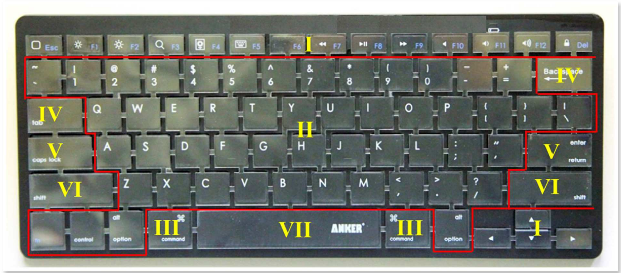
Supporting Figure S3 | Keys classification in the intelligent keyboard. The keys in the keyboards are classified into seven kinds according to their dimensions.
