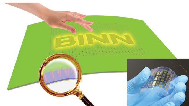
Figure 1. Schematic illustration of the flexible NW-LED-based pressure sensor array after applying a compressive strain. The device is based on a ZnO NW/p-polymer array. The inset is a photograph of the flexible device.
