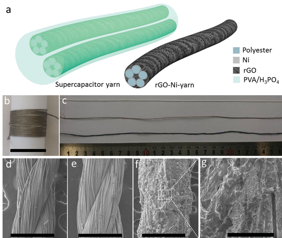
Figure 1. The fabrication of the yarn supercapacitor. a) A scheme of the all-solid-state symmetric yarn supercapacitor composed of two rGO-Ni-yarns in parallel. b) A photograph of a 1 m long Ni-coated polyester yarn. c) A photograph of pristine polyester yarn (white), Ni-coated yarn (silver), and rGO-Ni-yarn (black). Scanning electron microscopy (SEM) images of d) a pristine polyester yarn, e) an Ni-coated yarn, and f, g) an rGO-Ni-yarn. The scale bar is 3 cm for panel (b), 500 \mu\text{m} for panels (d–f), and 50 \mu\text{m} for panel (g).
