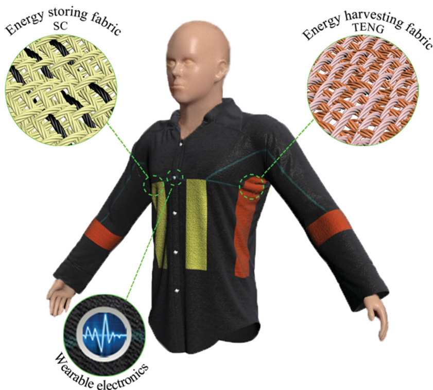
Scheme 1. Scheme of a self-charging power textile. It integrates the supercapacitor (SC) yarns as energy-storing fabrics, the triboelectric nanogenerator (TENG) cloth as energy-harvesting fabrics, and wearable electronics (e.g., button sensors).
