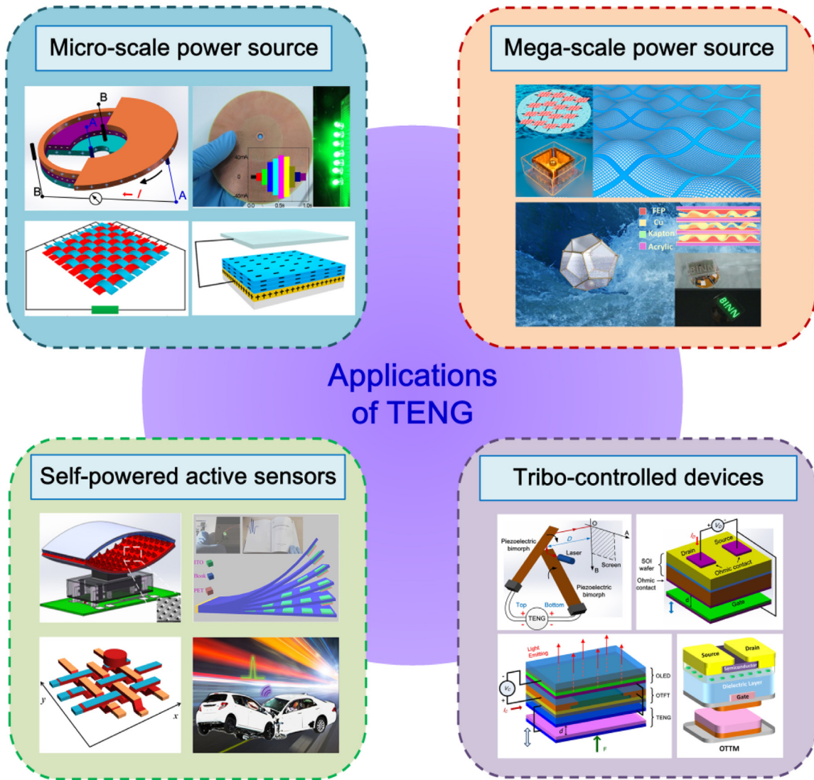
Fig. 14. Four applications of TENG. Besides the micro-scale power source, mega-scale power source and self-powered sensors, tribotronics is a new application of TENG as triboelectric-voltage-controlled (tribo-controlled) devices. Reprinted with permission from Refs. [35,77]. Copyright 2014 John Wiley & Sons, Inc. Reprinted with permission from Refs. [36]. Copyright 2015 Springer. Reprinted with permission from Refs. [37,67]. Copyright 2014 American Chemical Society. Reprinted with permission from Ref. [38]. Copyright 2016 Springer. Reprinted with permission from Refs. [49,57]. Copyright 2015 American Chemical Society. Reprinted with permission from Ref. [50]. Copyright 2016 Elsevier Ltd. Reprinted with permission from Ref. [54]. Copyright 2014 IOP Publishing Ltd. Reprinted with permission from Ref. [55]. Copyright 2014 Springer. Reprinted with permission from Ref. [56]. Copyright 2014 Elsevier Ltd. Reprinted with permission from Refs. [69,70]. Copyright 2015 John Wiley & Sons, Inc.
