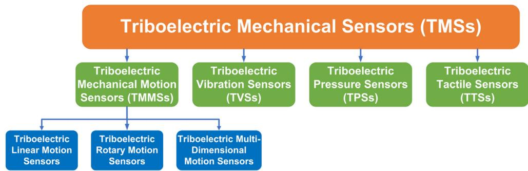
**Fig. 3.** The triboelectric mechanical sensors (TMSs) include four types of mechanical motion sensors, vibration sensors, pressure sensors and tactile sensors.
