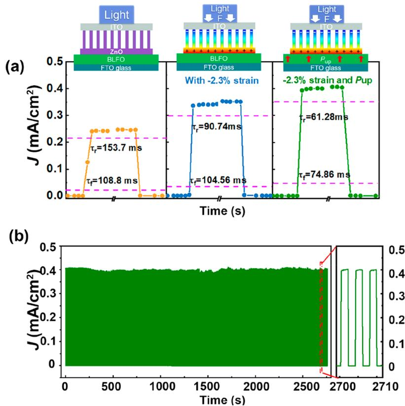
Figure 5. (a) Response time of the BLFO/ZnO heterojunction with different measurement conditions. (b) Durability test results of the BLFO/ZnO heterojunction with  $-2.3\%$  compressive strain and upward poling state under the illumination of 405 nm and power density of  $100 \text{ mW/cm}^2$ .
