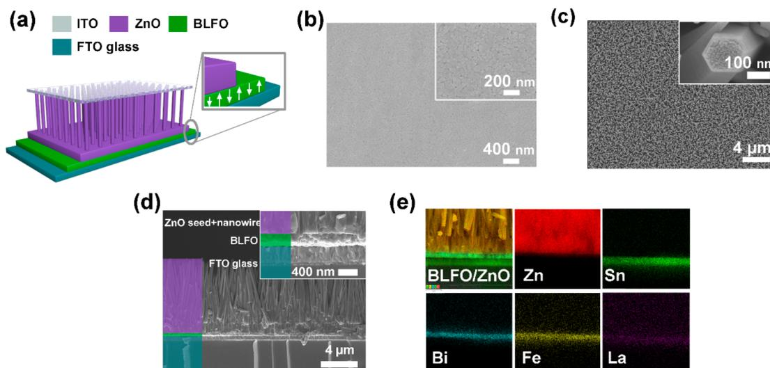
**Figure 1.** (a) Schematic structure of the BLFO/ZnO heterojunction. Top-view SEM images of the (b) BLFO film and (c) ZnO nanowire arrays, respectively. (d) Cross-section SEM image of the BLFO/ZnO heterojunction. Each inset (a–d) represents a locally enlarged view of the corresponding master graph. (e) EDS elemental maps for the interfaces of the heterojunction.
