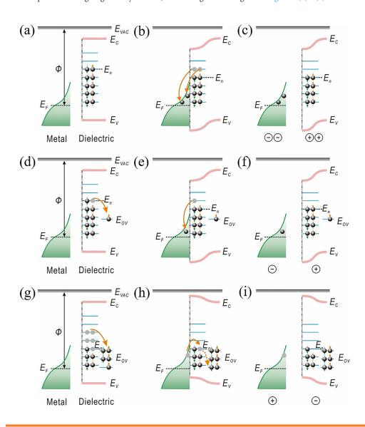
**FIG. 4.** Surface states model for explaining charge transfer between the metal and dielectric after (a)–(c)  $T_1$  annealing. (d)–(f)  $T_2$  annealing. (g)–(i)  $T_3$  annealing.  $\Phi$ , metal work function;  $E_{\rm F}$ , Fermi level;  $E_{\rm VAC}$ , vacuum level;  $E_{\rm C}$ , conduction band;  $E_{\rm N}$ , reutral level of surface states;  $E_{\rm V}$ , valence band;  $E_{\rm OV}$ , level of oxygen vacancy;  $T_1 < T_2 < T_3$ .
