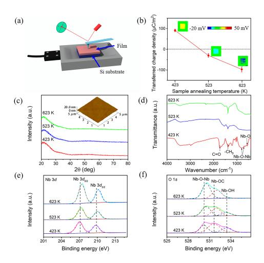
**FIG. 1.** (a) The generation of the triboelectric charges on the film surface by using the KPFM mode. (b) The triboelectric charges under the room temperature on  $\mathrm{Nb}_2\mathrm{O}_5$  films after the samples being annealed at different temperatures. (c) XRD results of the films and inset is the surface topography of the film annealed at 623 K. (d) FTIR results of the films. XPS results of (e) Nb 3d and (f) O 1s of the films.
