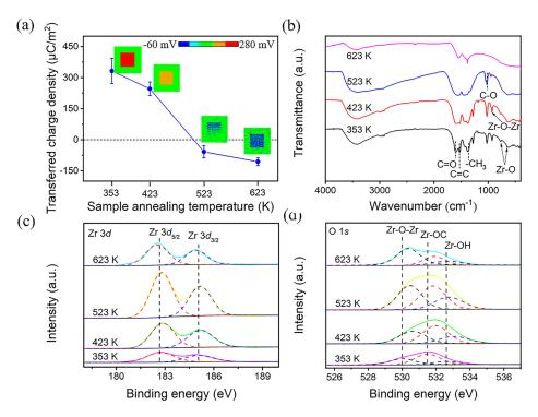
**FIG. 3.** (a) The triboelectric charges under the room temperature on  $ZrO_2$  films after treated at different temperatures. (b) FTIR results of the films. XPS results of Zr 3d (c) and O 1s (d) of the films.
