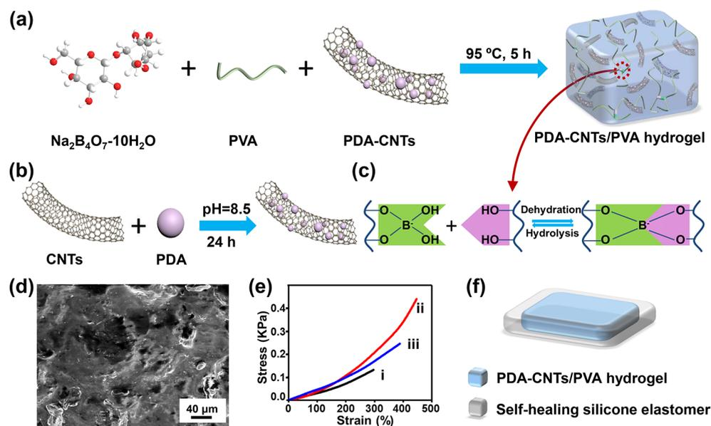
**Figure 1.** Illustration and characterization of the MF-TENG. (a) Preparation process of the PDA-CNTs/PVA hydrogel; (b) Schematic diagram of the PDA modification of CNTs; (c) Self-healing mechanism of the PDA-CNTs/PVA hydrogel; (d) SEM image of the PDA-CNTs/PVA hydrogel; (e) Stress–strain curves of (i) pure PVA, (ii) the original PDA-CNTs/PVA hydrogel, and (iii) the self-healed PDA-CNTs/PVA hydrogel; (f) Schematic structure of the MF-TENG.
