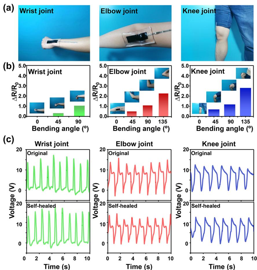
**Figure 3.** Application of the MF-TENG to different joints of a human body for large-scale human motion. (a) Photos of the MF-TENG attached to different joints of the human body; (b) Relative resistance variations of the MF-TENG attached to the wrist, elbow, and knee joints motion at different bending angles; (c) Open-circuit voltage of the original and self-healed MF-TENG for the wrist, elbow, and knee joints motion at the ultimate bending angle, respectively.
