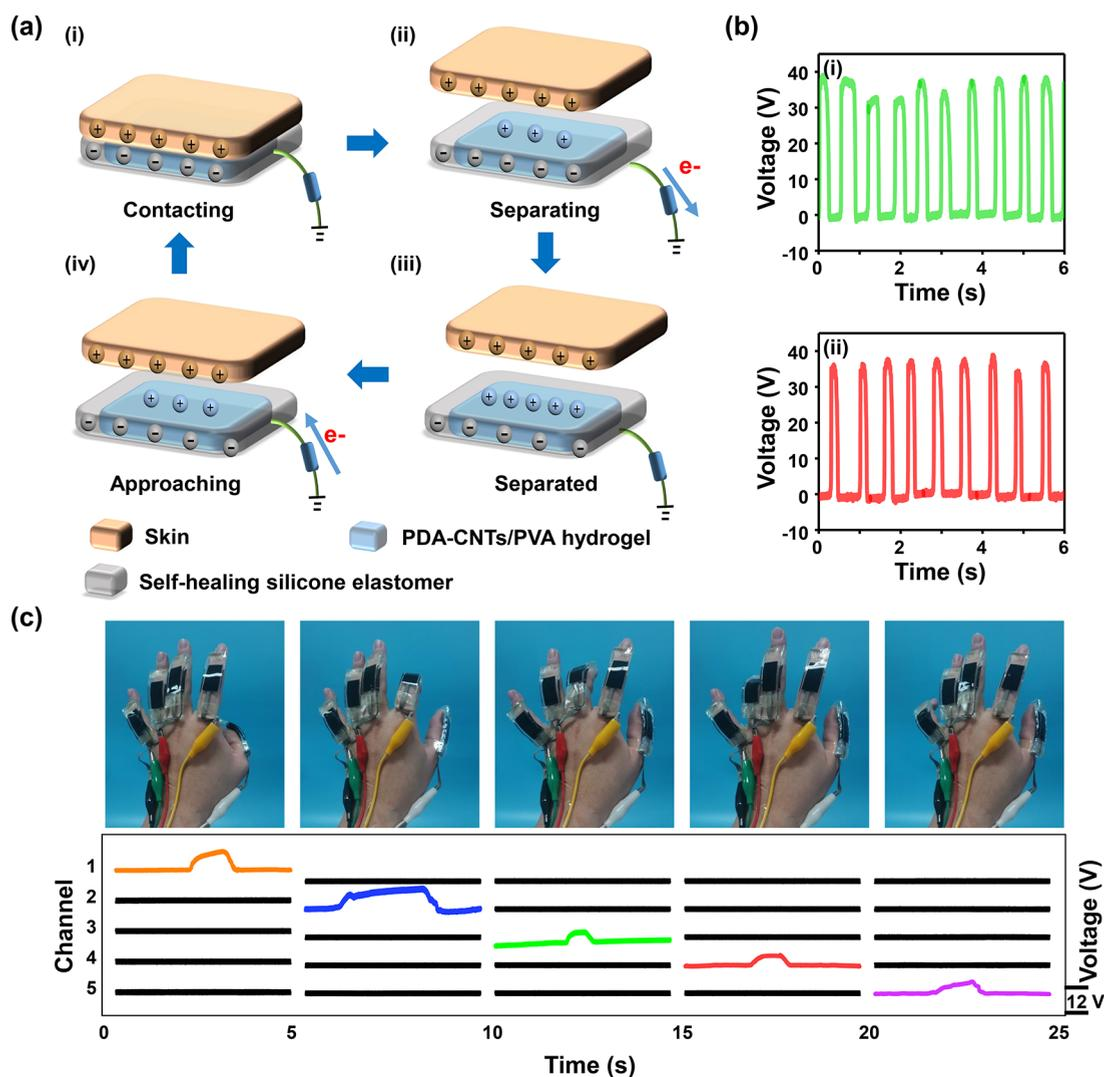
**Figure 2.** (a) Schematic illustration of the working mechanism of the MF-TENG in single-electrode mode; (b) Open-circuit voltage of (i) the original and (ii) the self-healed MF-TENG; (c) Real-time responses of the bending of fingers acquired via five channels made of the MF-TENG.
