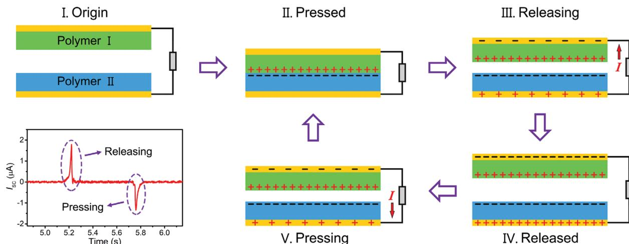
**Figure 2.** Sketches illustrating the working principle of the TENG in contact-separation mode.
