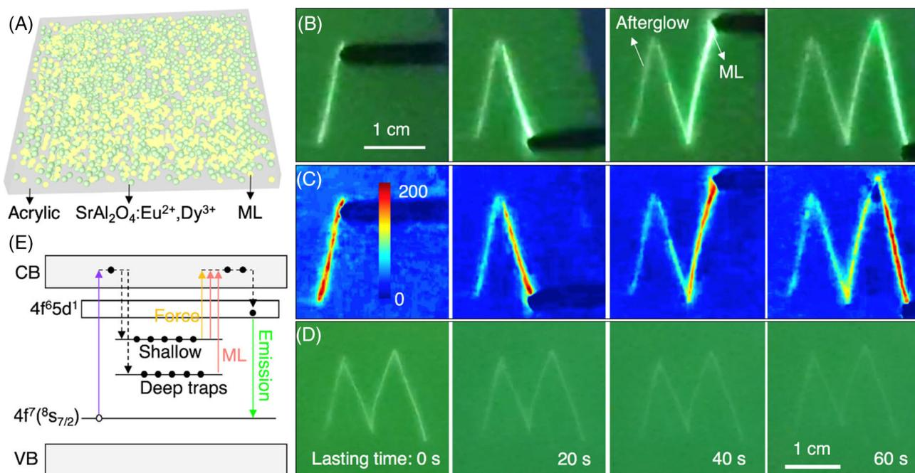
**FIGURE 2** Visual sen-memory of the pressure. (A) Schematic of the device in conjunction of ML hybrids and phosphor embedded in acrylic matrix for the visual sen-memory of the pressure. (B,C) The photographs and the corresponding intensity maps of the device during the sen-memory process of the applied force. (D) The afterglow images of the device after the removal of the applied force. (E) Schematic illustration of the sen-memory mechanism
