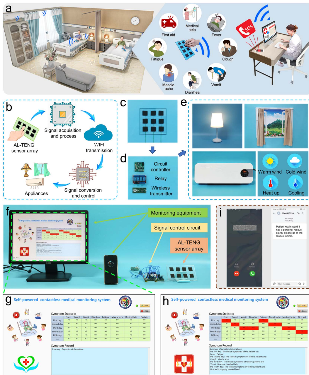
Fig. 5 Application of the AL-TENG in smart ward and medical monitoring. (a) Schematic diagram of the TENG-based self-powered smart ward. (b) Schematic diagram of the self-powered smart ward system. (c)–(e) Demonstration photographs of the wireless control system based on the AL-TENG: (c) AL-TENG sensor array, (d) signal control circuit, and (e) smart appliances. (f) Demonstration of the self-powered contactless medical monitoring system. (g) and (h) Operating interface of the self-powered contactless medical monitoring system. (i) Screenshot of the mobile phone showing the emergency calls and messages.
