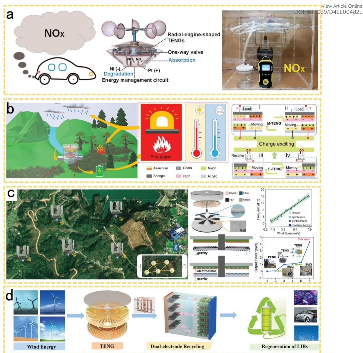
Fig. 14 The application of F-TENG in Environment Protection. (a) NO x absorption and degradation system based on TENG. 175 (b) Water-flow energy harvesting and intelligent forest monitoring by the CEMA-TENG. 177 (c) A self-powered wireless sensing network to achieve long-term and wide-area local temperature, humidity, and atmospheric pressure monitoring. 180 (d) Self-powered system for recycling used LFP batteries by capturing wind energy through TENG. 186
