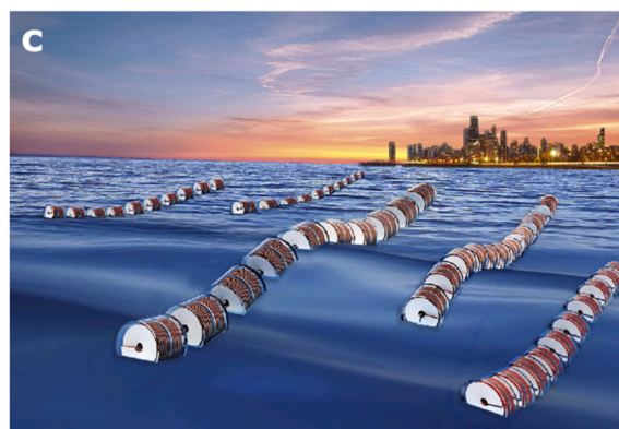
Fig. 7. Wave energy scavenging. a, Floating nets of nanogenerators to scavenge renewable wave energy. Reprinted with permission [197]. Copyright 2017, Springer Nature. b, TENGs' applications for deployment at sea. c, TENG-based wave energy harvester using an anaconda-shaped spiral multi-layered structure. Reprinted with permission [205]. Copyright 2021, Cell Press.
